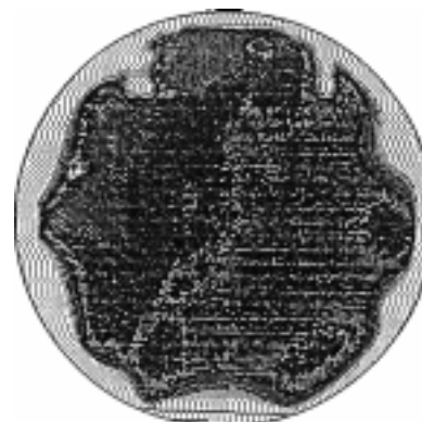
Fig. 3. MCLT map of As implanted wafer showing contamination introduced from clamps securing the wafer in the ion implanter.
